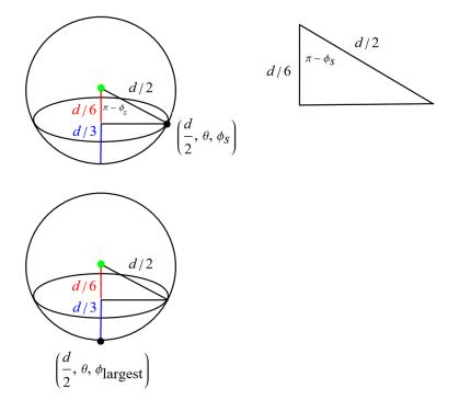
Use trigonometry to determine the shortest value of  $\phi$ ,  $\phi_S$ .
